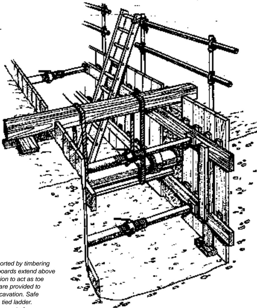
*This excavation is supported by timbering and props. The poling boards extend above the edge of the excavation to act as toe boards and guard rails are provided to prevent falls into the excavation. Safe access is provided by a tied ladder. Exposed services are supported.*
